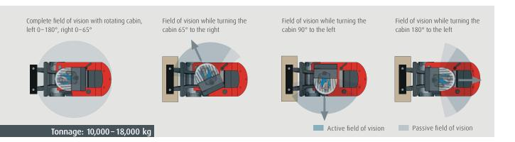
The optional rotating cab is a special feature of the Linde H100 to H180 heavy-duty trucks and allows the driver to rotate the entire cab in infinitely variable stages up to an
