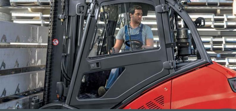
Operating the rotating driver's workstation is simple and intuitive. Using a single handle, the entire workstation including the seat with operating unit, the steering wheel and the pedals can be adjusted to the required position. In addition, the rotating driver's workstation can be swivelled in intermediate stages.
